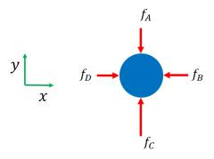
4. The static blue disk-shaped particle shown above is under influence of four diametrically oriented contact forces  $f_i$ . If we know that the dyadic product  $\otimes$  is defined as
